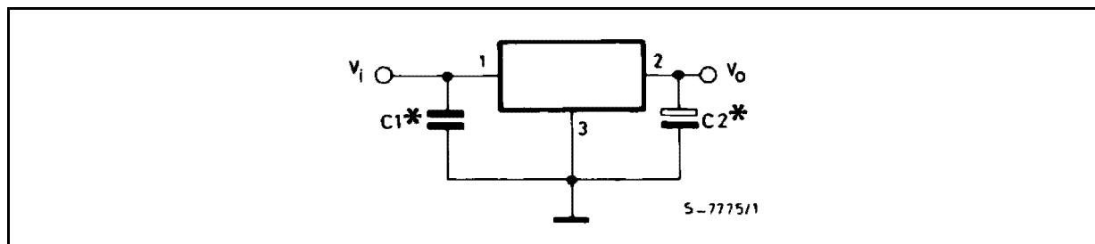
(\*) Note : C1 and C2 are only needed if the load capacitance exceeds 1000 pF, Recommended values are C1 = 0.1 µF and C2 ≥ 100 µF.
