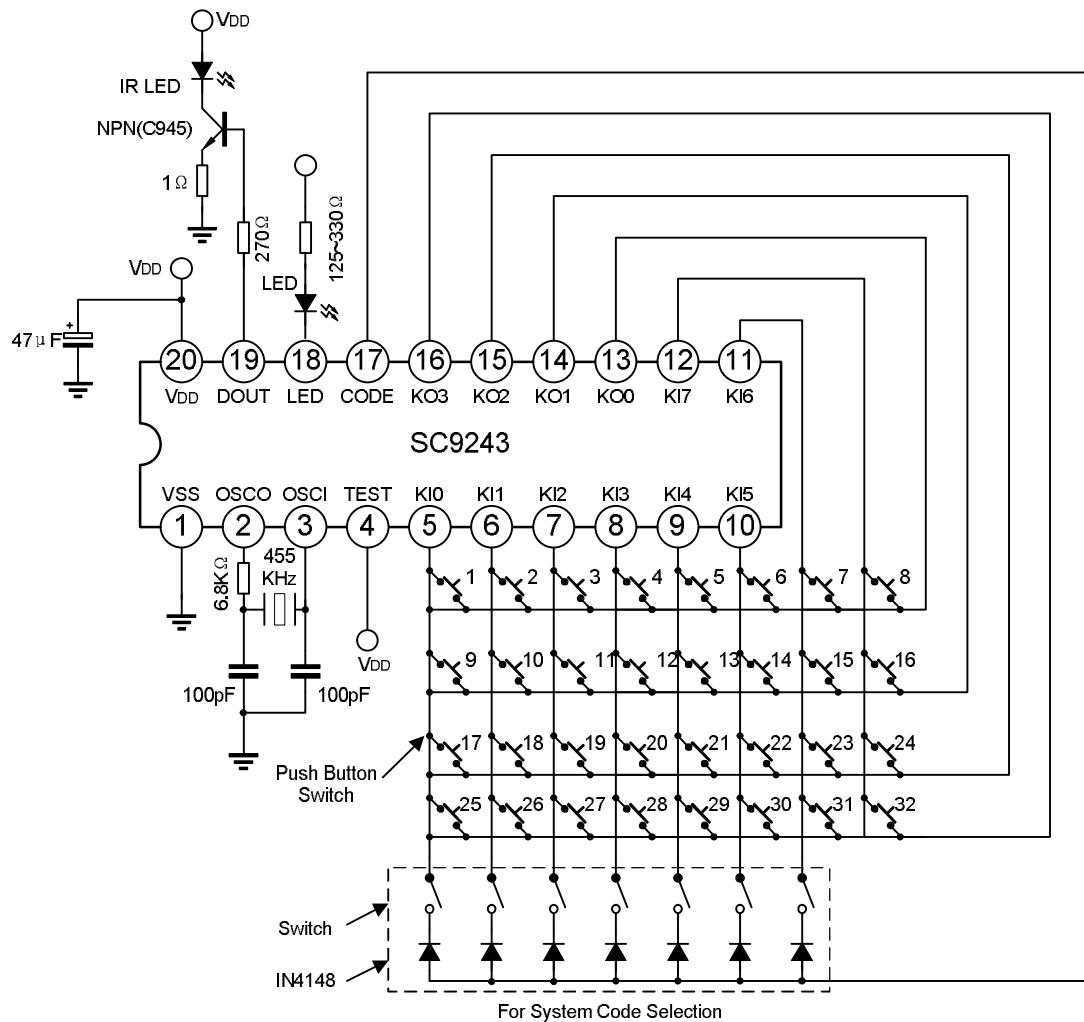
PCB WIRE LAYOUT SCHEMATIC
