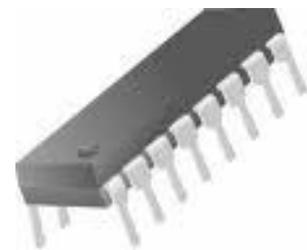
The circuit is ideally suited for communications, instrumentation, and function generator applications requiring sinusoidal tone, AM, FM, or FSK generation. It has a typical drift specification of 20ppm/°C. The oscillator frequency can be linearly swept over a 2000:1 frequency range with an external control voltage, while maintaining low distortion.
