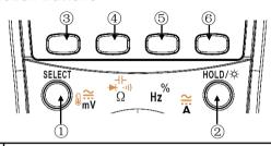
Selects alternate measurement modes on a rotary switch setting, including:
