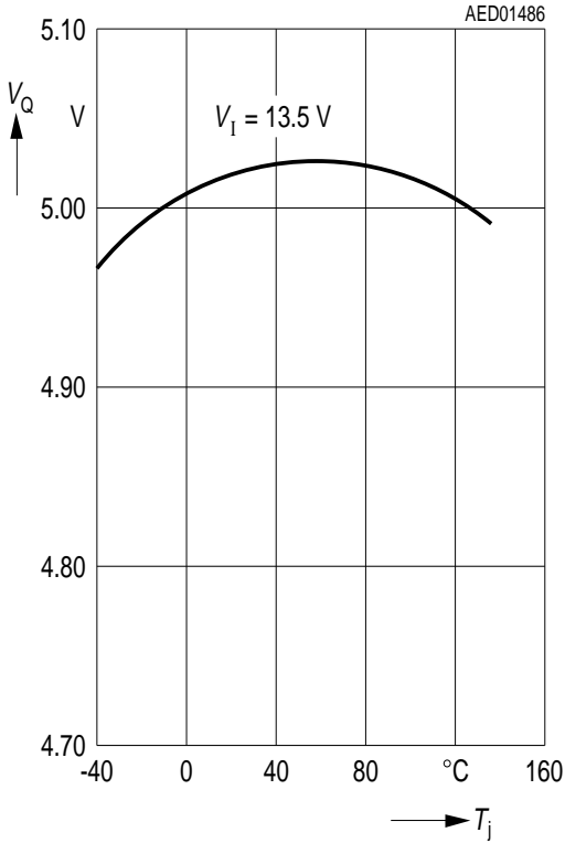
Output Voltage V_Q versus Temperature T_j
