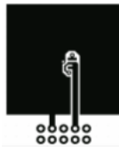
a) 78^\circ\text{C/W} when mounted on a 1\text{ in}^2 pad of 2 oz copper
