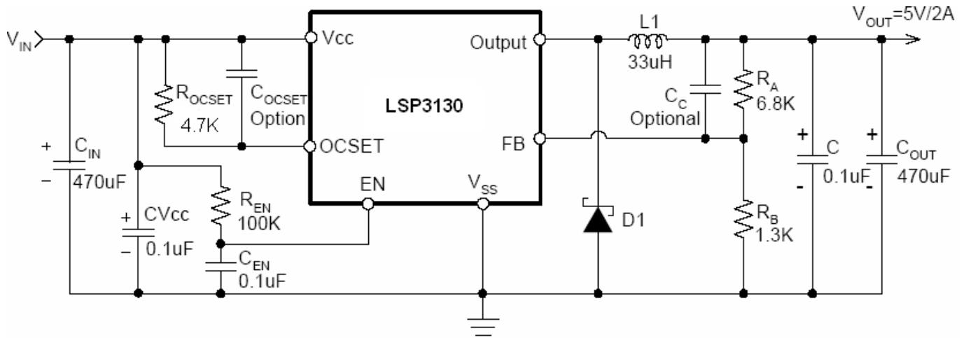
Note1:  $C_{IN}/C_{OUT}$  can be Electro capacitor or Tan capacitor; The typical  $C_{IN}$  Electro capacitor is 470uF/35V, the typical  $C_{IN}$  Tan capacitor is 100uF/35V; The typical  $C_{OUT}$  Electro capacitor is 470uF/16V, the typical  $C_{OUT}$  Tan capacitor is 22uF/16V;
