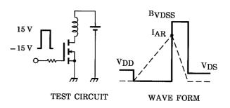
$$\begin{aligned} &RG = 25~\Omega \\ &V_{DD} = 25~V,~L = 221~mH \end{aligned} \qquad EAS = \frac{1}{2} \cdot L \cdot I^2 \cdot \left(\frac{BVDSS}{BVDSS - V_{DD}}\right)$$
