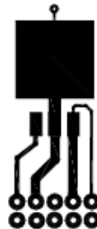
b. 96\text{ }^\circ\text{C/W} when mounted on a minimum pad of 2 oz copper.
