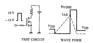
$$\begin{aligned} R_G &= 25~\Omega \\ V_{DD} &= 25~V,~L = 272~\mu H \end{aligned} \qquad EAS &= \frac{1}{2} \cdot L \cdot I^2 \cdot \left( \frac{BVDSS}{BVDSS - VDD} \right) \end{aligned}$$
