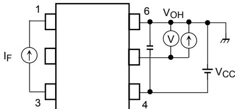
**Test Circuit 4: V<sub>OL</sub>**
