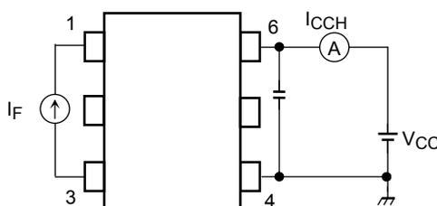
**Test Circuit 6: I<sub>CCL</sub>**
