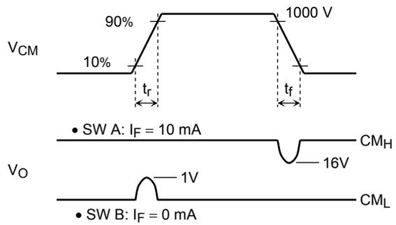
$$C_{ML} = \frac{800 \text{ V}}{t_f (\mu\text{s})}$$
