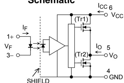
A 0.1  $\mu\text{F}$  bypass capacitor must be connected between pins 6 and 4. (See Note 6.)
