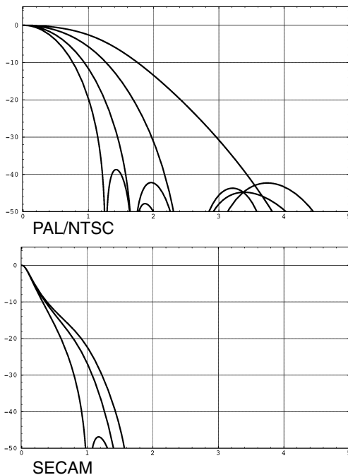
Fig. 2-5: Frequency response of chroma filters
