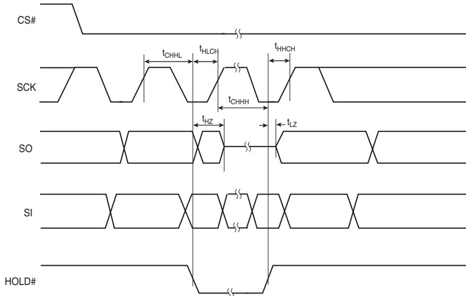
**Figure 18.5** Write Protect Setup and Hold Timing during WRR when SRWD = 1
