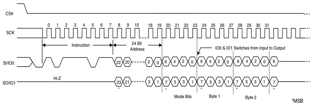
Figure 9.6 Continuous Dual I/O High Performance Read Instruction Sequence
