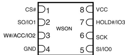
**Figure 2.4** 8-contact WSON Package (6 x 8 mm)
