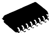
Outline 16P2N-A(FP) 1.27mm pitch 300mil SOP (5.3mm × 10.1mm × 1.8mm)
