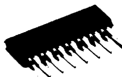
Outline 14P5A(L) 1.27mm pitch 325mil ZIP (2.8mm × 19.0mm × 6.3mm)
