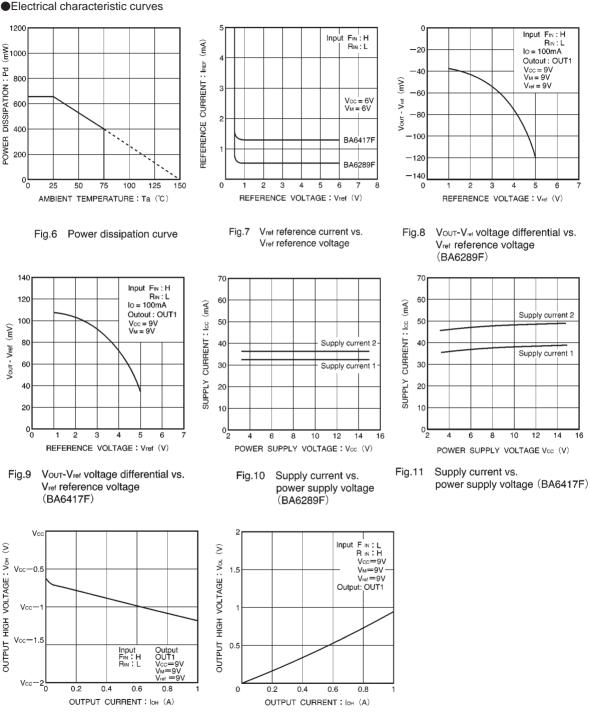
Fig.12 Output high level voltage vs. output current
