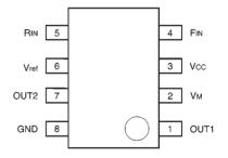
Fig.1 Pin assignments
