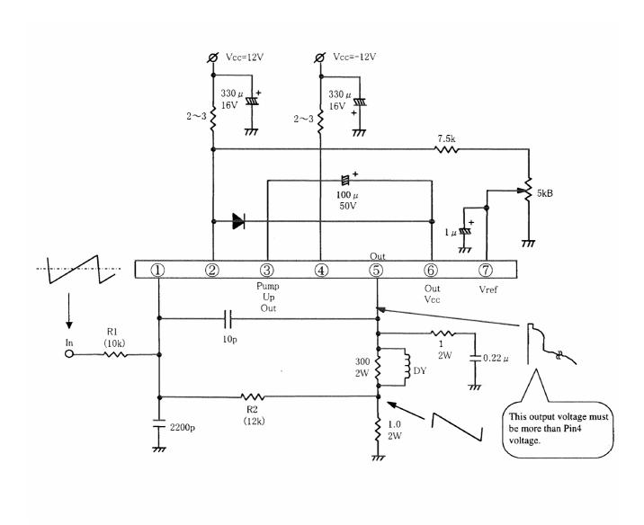
In order to get required gain, it is necessary to adjust the R1 and R2.
