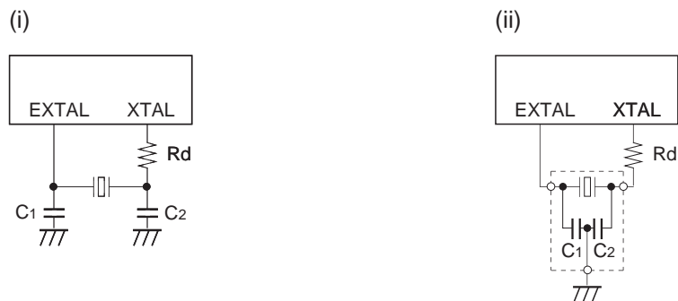
Fig. 13. Recommended Oscillation circuit
