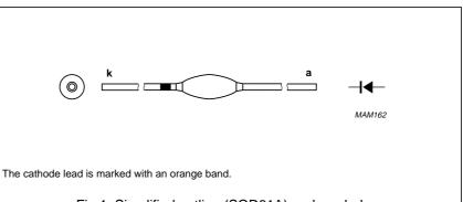
Fig.1 Simplified outline (SOD61A) and symbol.
