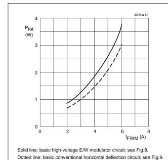
Curves include power dissipation due to switching losses.
