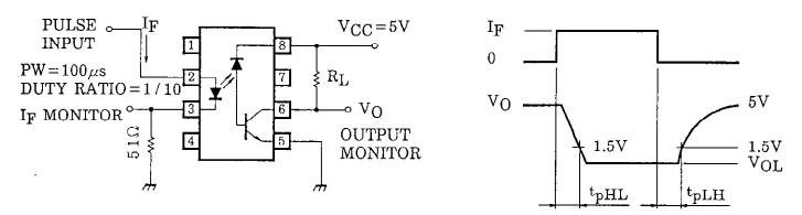
TEST CIRCUIT 2 : Common Mode Noise Immunity Test Circuit
