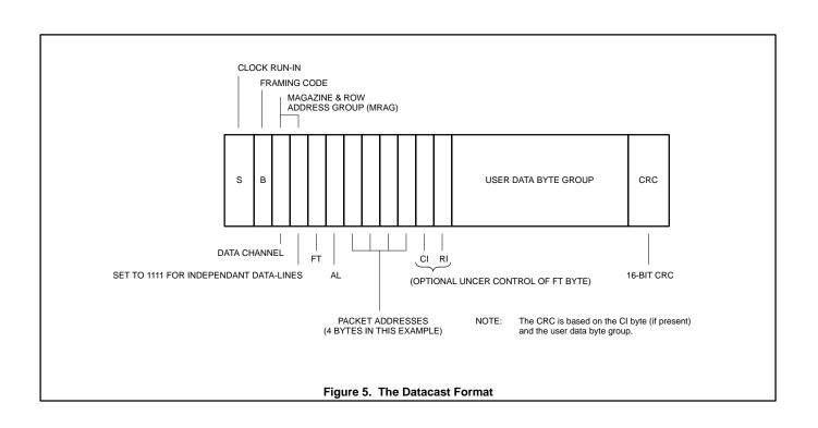
If the Repeat Indicator is in use, the software should arrange temporary buffering of the multiple transmissions of data and make a choice on the basis of the comparisons, plus the CRC check, as to which data is valid. The data must only be sent to the host once from the decoder if the proper data sequence is to be preserved. The Repeat Indicator is used by the software routine to ensure that repeated data is not sent out to the host again. A simplified flow chart can be found in Figure 6.
