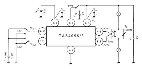
Note: Calibrate I<sub>OUT</sub> to 0.2/0.4 A by R<sub>L</sub>.
