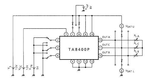
Note: Calibrate  $I_{OUT}$  to 0.4 / 1.0A by  $R_{LA}$ ,  $R_{LB}$  and  $R_{LC}$ .
