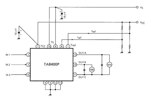
Note: Pin (16) is required to connect to pin (9).
