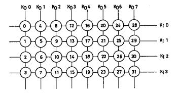
Multi-press of key No. 20 and one of key No. 21, 22, 23 may be done, with no priority given in key entry. When the two keys are kept pressed, a series of pulses will be output according to each key entry. If multi-press of keys which are not allowed multi-press is done, no output will be delivered.
