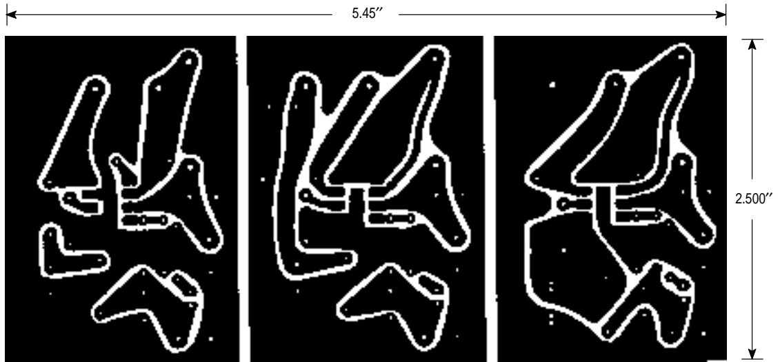
(Top view, copper foil as seen through the board from the component side)
